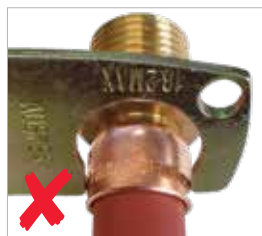
Fitting has been under crimped
