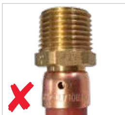
Witness hole not completely filled
