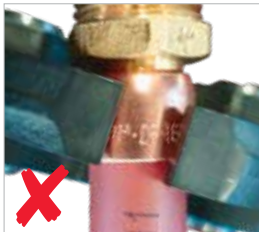
Jaw not square on the crimp ring
