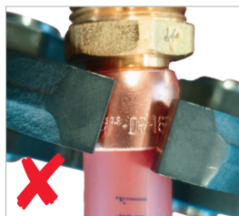
Jaw not square on the crimp ring
