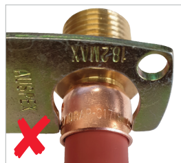
Fitting has been under crimped
