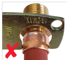
Fitting has been under crimped
