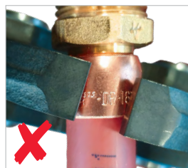
Jaw not square on the crimp ring
