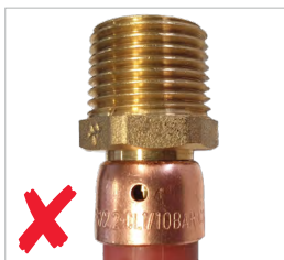
Witness hole not completely filled
