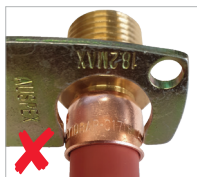
Fitting has been under crimped
