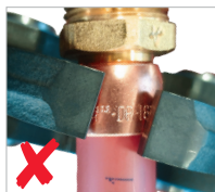
Jaw not square on the crimp ring
