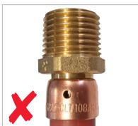
Witness hole not completely filled
