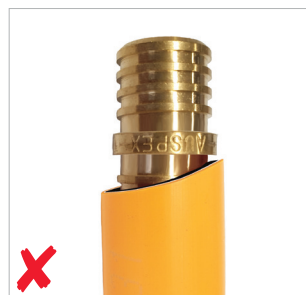
Pipe badly cut and not square to fitting
