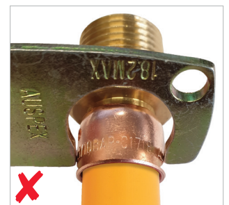
Fitting has been under crimped
