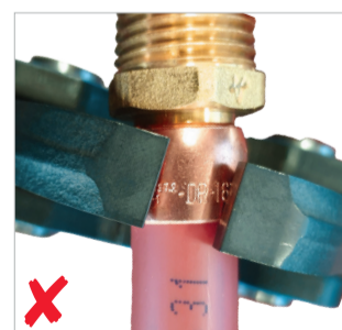
Jaw not square on the crimp ring
