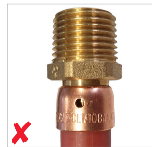
Witness hole not completely filled
