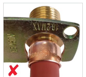
Fitting has been under crimped
