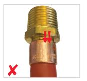
Fitting has been double crimped
