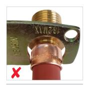
Fitting has been under crimped
