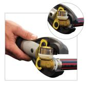
Press the switch mechanism until the joint is completed. Press the back end of the jaws and remove the completed joint.
