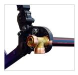
When using a battery tool, ensure the tool has fully closed and released indicating a completed joint.
