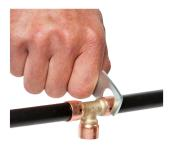
If the gauge experiences any interference the joint is under crimped. The tool should then be adjusted. Do not double crimp.
