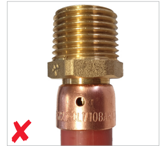
Witness hole not completely filled
