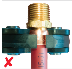
Jaw not centered on the crimp ring
