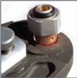
Step 14c. Crimp fitting
